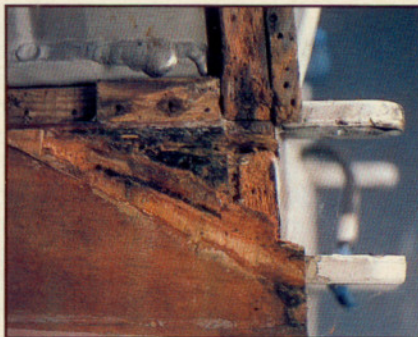
Front seat rail obstructs landing gear pump, complicating service and maintenance (left). Aluminum corrosion is not a concern with a Viking wood spar; decay-producing fungi is (right).
